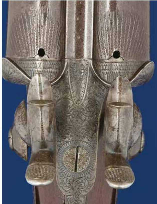
A 12-bore pinfire gun by Dougall on his 'Lockfast' patent of 1860. Pin-holes in the barrels allowed the hammers to strike the protruding pins and detonate the charge.
