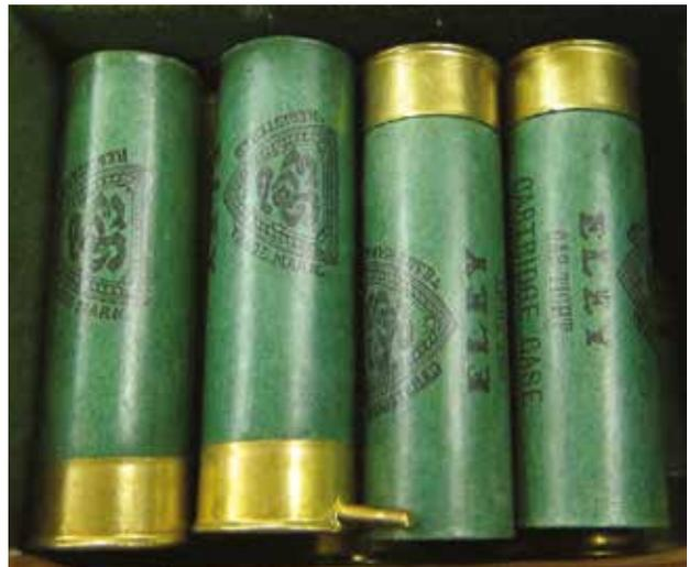
Pinfire cartridges put the detonation charge, the main powder charge and the shot charge into one portable container. For the first time, a new unit could replace a spent one in a second.
