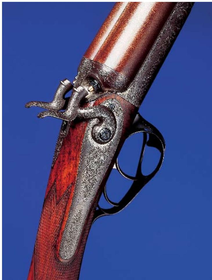
Above left: a conventional bar-action hammer gun circa 1880, by Gallyon. On the right is a late 1870s back-action hammer gun by Purdey. Note the isolated lock plates.
