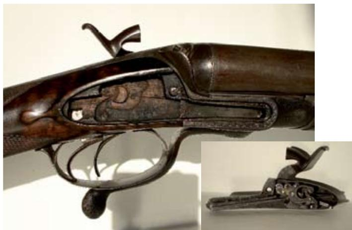
These pictures illustrate the internal components of the bar-action hammer lock (inset) and the recesses cut into the wood and the bar of the action to accommodate the internal mechanism. The gun has re-bouncing locks and is by J. Thompson and dates from the late 1870s.
