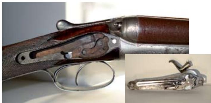
Here can be seen the internal components of a back-action hammer lock (inset) and the recess in the stock cut away to receive the mechanism. This is an 1885 Holland & Holland with rebounding locks.
