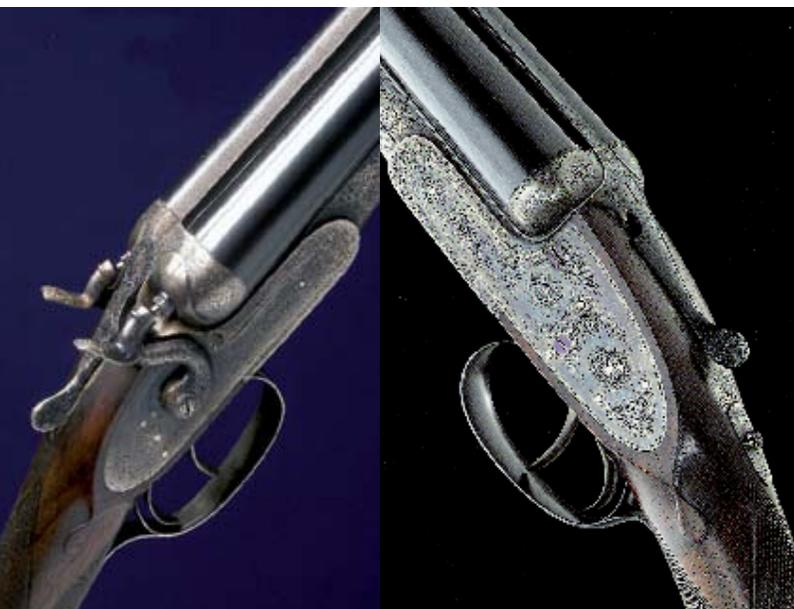
Left: Purdey pigeon hammergun. Right: Purdey hammerless sidelock. Both guns are twelve bores and use bar-action sidelocks.
